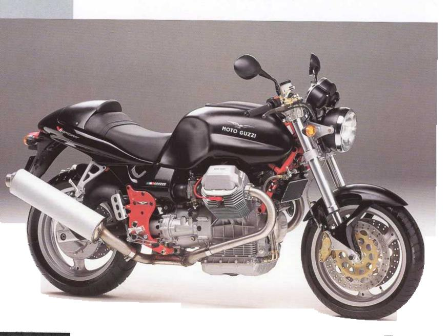
Based on the classic steel single rectangular box section with structural engine block, the frame has also been given special attention. The steering angle, one degree sharper than the preceding Sport Corsa model (26° to 25°), make the V11 Sport the best handling Guzzi's ever produced.
